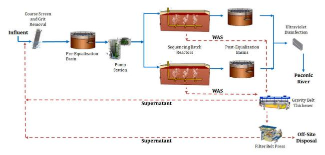
Figure 4: SBR System as Installed in 2000
