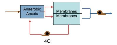
Figure 3: Batch-Style MBR for Maximum BNR
