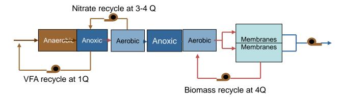
Figure 2: Typical Conventional Flow-Through MBR for Maximum BNR
