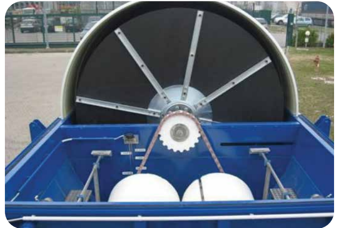
Internal view of the RBC and cloth media drum filters.
