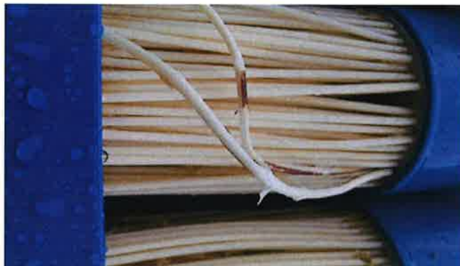
Figure 12. Fibers Sliced by the Lower Module Frame
