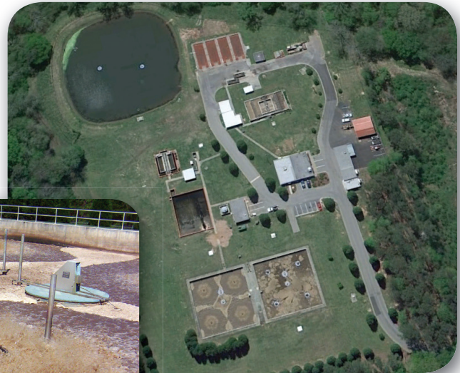
Aerial view showing the 2-basin AquaSBR ® system; a closeup of the system in operation is shown to the left.
